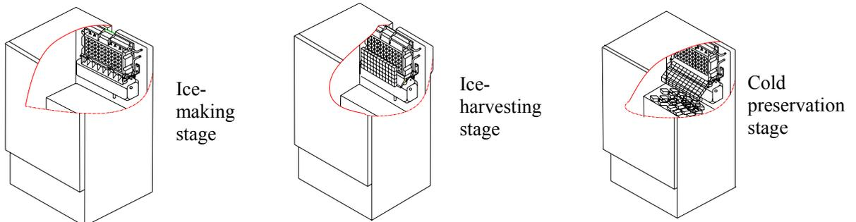
2. After three minutes, the machine will automatically go into the ice-making stage, and the sound of flowing water will be heard.
