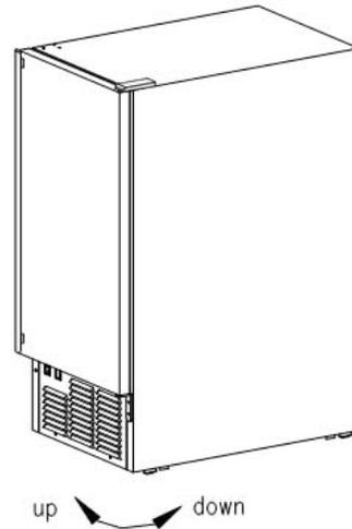
1. Place a carpenter's level on top of the product to see if the ice maker is level from front to back and side to side.
